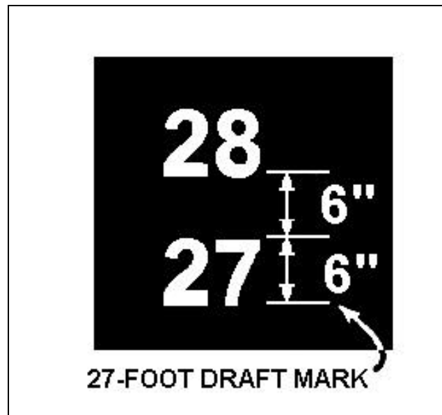
Figure 3-8. Draft Numbers Showing Foot Draft Mark
