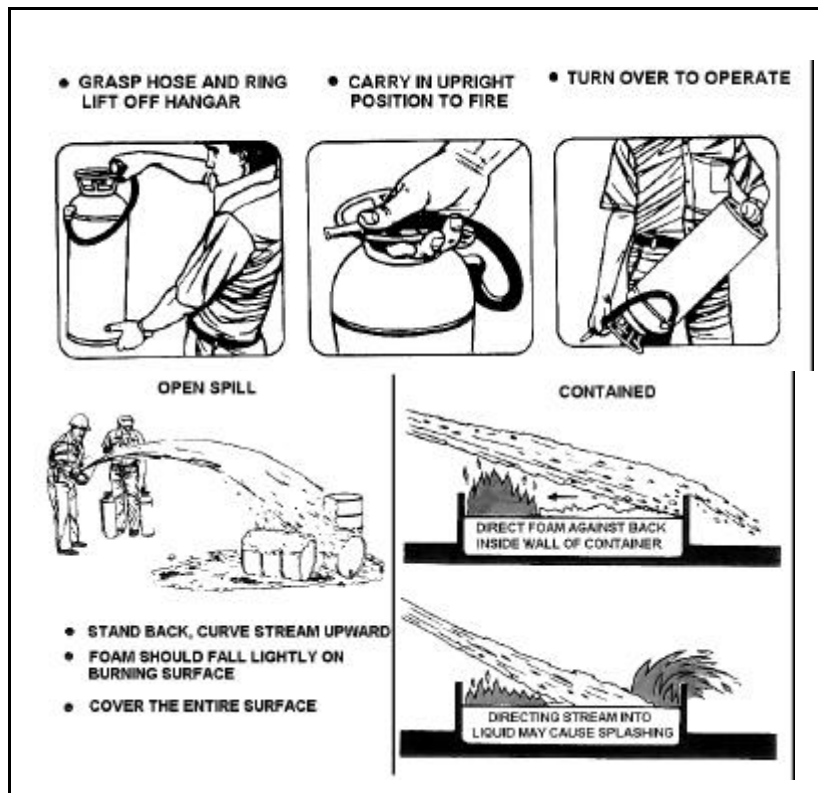
Figure 11-20. Operating a Foam Extinguisher on a Flammable Liquid Fire
