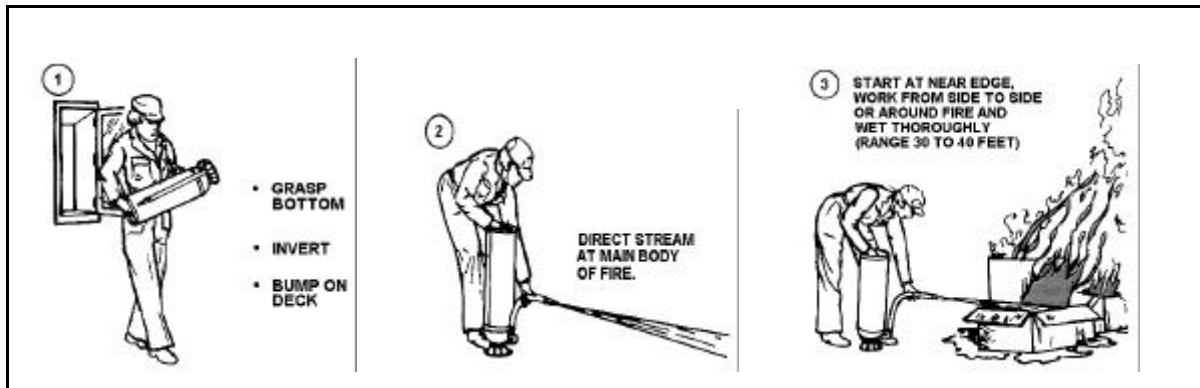
Figure 11-18. Using the Cartridge-Operated Extinguisher
